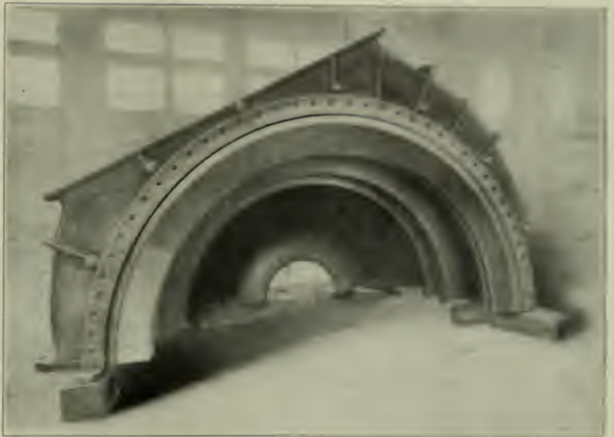
FIG. 17 UPPER HALF OF EXHAUST END OF CASING
